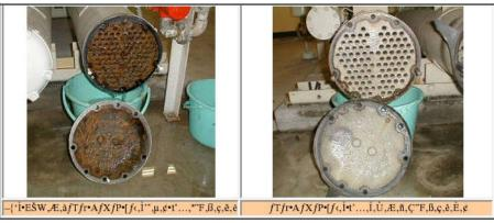
Compressor Heat Exchange Tubes in Japan before and after installation of EcoBeam XL
